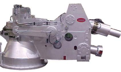
The opening mechanism is actuated by a hydraulic cylinder and features an over-center spring assembly, providing automatic pressure relief. Once open, the valve lid is positioned out of the gas flow.
