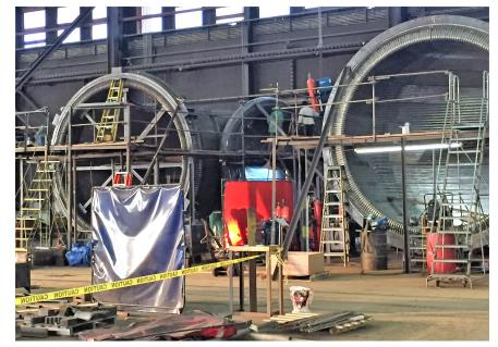
Munroe's application process produces a very consistent overlay thickness that is completely bonded to the tubes. This innovation eliminates overlay spalling, ensures a proper weld joint with the desired strength and solves many other fabrication issues.
