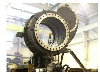
Manufactured from stainless steel, the plate will feature rubber seats on both the open and closed rings. The swinging goggle plate is electro-mechanically operated
