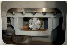
Hydraulic cylinders replace the traditional mechanical function for tilting the revolving chute.
