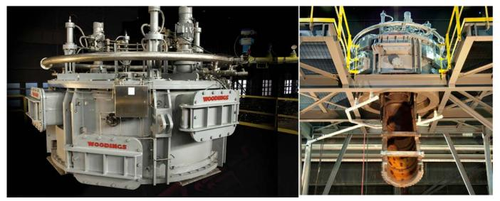
Hydraulic cylinders replace the traditional mechanical function for tilting the revolving chute.
