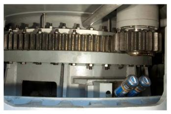
Rotation of the chute is accomplished with a simple gearbox and electric motor.
