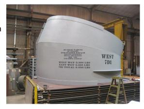
Munroe was tasked with the fabrication of three large duct sections each weighing between 6600 and 8900 pounds.
